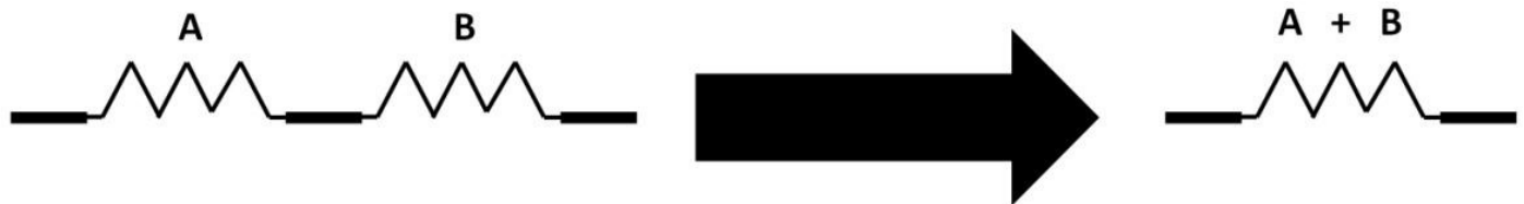
Figure 1.11: Series resistor rule
